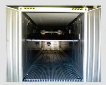
The new and improved AFE-30 false ceiling allows for even faster blast freezing by ensuring that the maximum airflow is pulled across your product. This ensures quicker cooling and less overall power use.
